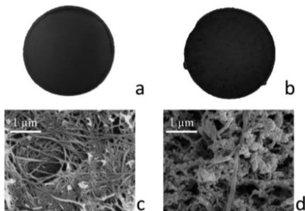
Fig 5. Final appearance of (a) neat SWCNT-BP and (b) MTV-MOF/SWCNT-BP. The average diameter of membranes was  $38 \pm 1$  mm. SEM images of (c) SWCNT-BP and (d) MTV-MOF/SWCNT-BP unveiling MTV-MOF micrometer particles as aggregates of smaller nanosized primary particles.
