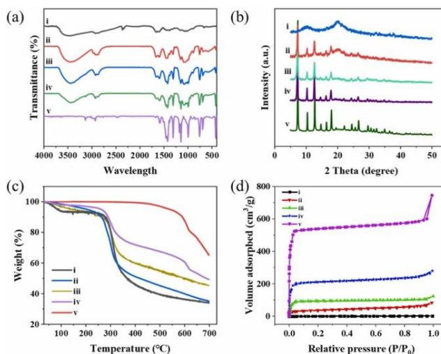
Fig. 1. (a) FT-IR spectra, (b) PXRD patterns, (c) TGA curves and (d) N<sub>2</sub> adsorption/ desorption isotherms of CS (i), CS-ZIF-8-1:1 (ii), CS-ZIF-8-2:3 (iii), CS-ZIF-8-1:2 (iv) and ZIF-8 (v). [31]
