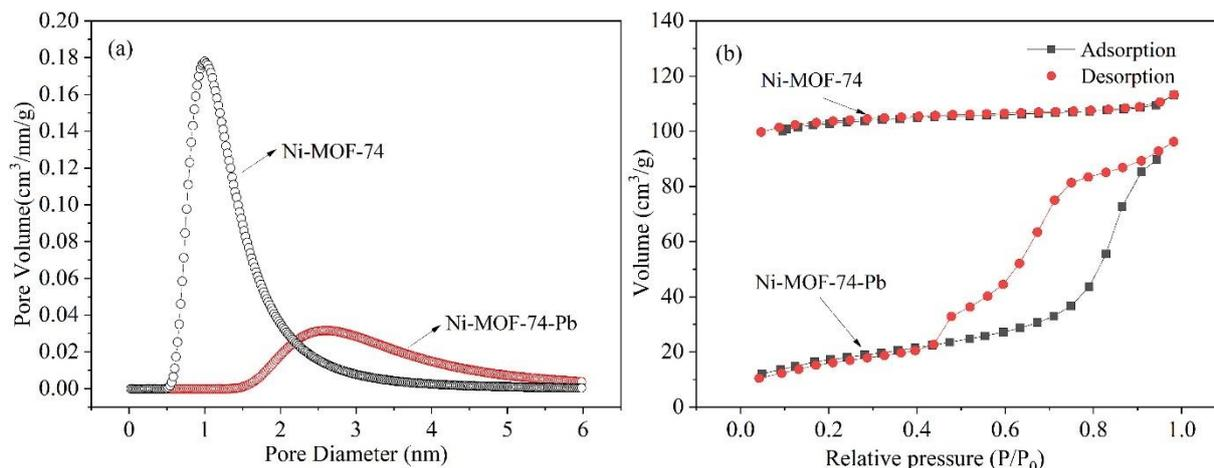
Fig7. (a) pore size distribution curves of Ni-MOF-74 and Ni-MOF-74-Pb, (b) N<sub>2</sub> adsorption/desorption isotherms. [43]
