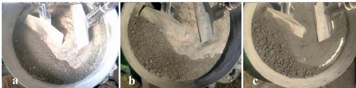
Fig. 4: Granulation process for artificial aggregates
